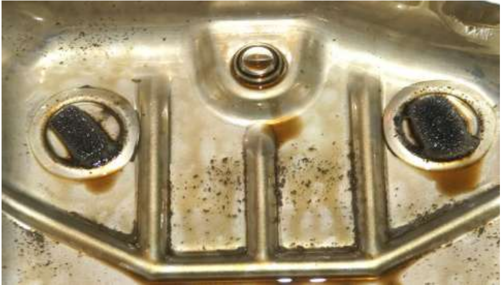
Magnets showing amount of debris attached
